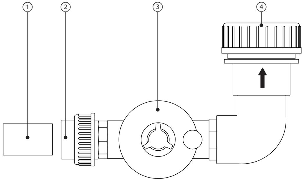
Figure 2-3 Filling module with float valve
