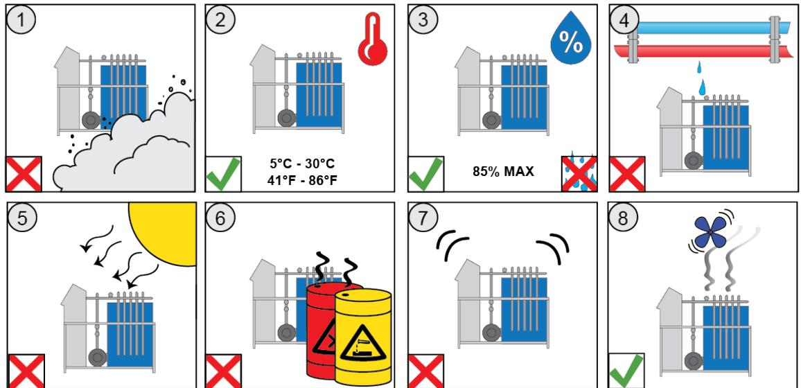
Figure 4-1: Illustrations showing installation requirements
