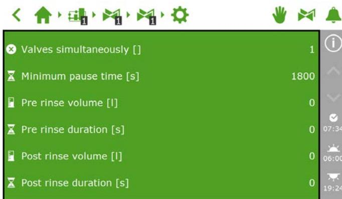
Figure 6-11: The settings associated with pre-flushing and post-flushing
