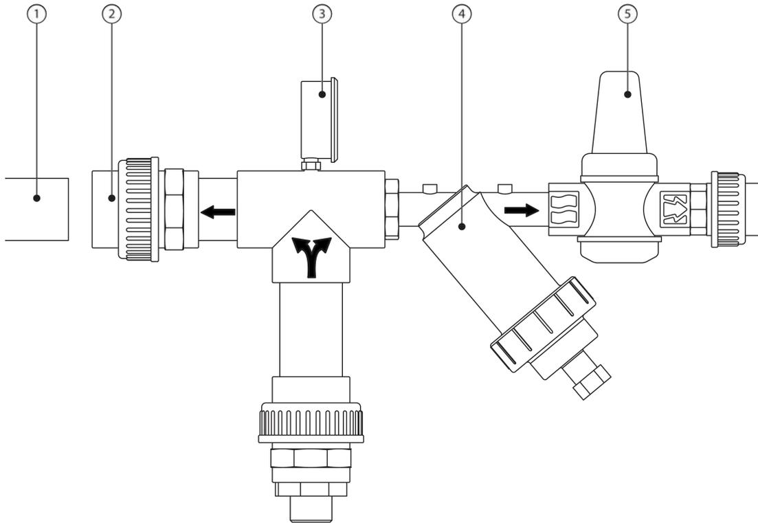
Figure 2-4 Pressure module with filter
